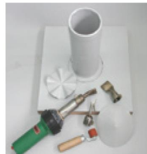
Hand Welding Guns and Prefabricated Parts
